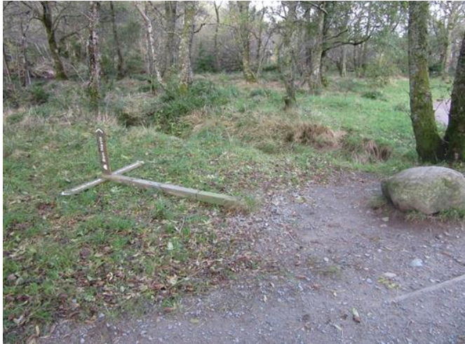
Figure 15. Finger post sign snapped at the base (Rangers, 2021)
